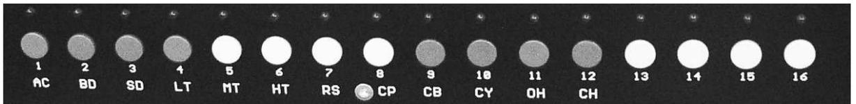
For example, if the Length Button and the button at step 12 is pressed, the pattern will be 12 steps long; after running through the first 12 steps, the pattern will repeat. The pattern length will stay the same even after changing to another mode. The unplayed steps after the last step remain in memory.
