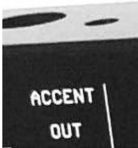
The Accent Out is primarily intended to be used to control an analog synthesizer with a gate input.
