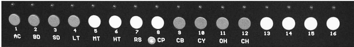
The active pattern will be indicated by a blinking LED above the corresponding button, and will start to play after the end of the last pattern. The pattern will repeat continuously as in Pattern Play Mode. By pressing the Write/Next button, you can set the current pattern as the first pattern in the Track.
