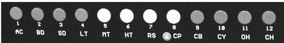
If you hold the Clear button while holding one of the instrument buttons for a longer period, that instrument will be erased from all of the steps the sequencer passes through during the time the buttons are held.
