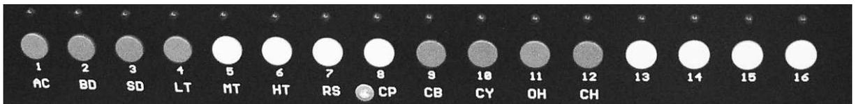
For example, if the Length Button and the button at step 12 is pressed, the pattern will be 12 steps long; after running through the first 12 steps, the pattern will repeat. The pattern length will stay the same even when changing to another mode. The unplayed steps after the last step remain in memory.
