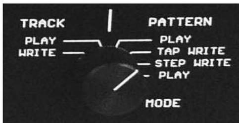
In this mode, unlike as in Pattern Tap Write Mode, you can only playback and edit a single pattern. The pattern to be edited depends on the pattern playing at the moment the mode is changed. This pattern will continue to play when the mode is switched back.
