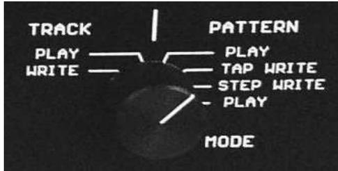
The sequencer runs continuously in all six modes. You can switch between modes while the sequencer is running; the switch takes place after the last step of the current pattern has been played.
