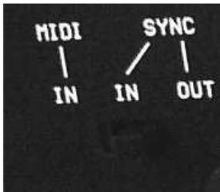
A Sync-out Signal will be generated at the Sync socket for other devices that have a Sync-In socket.
