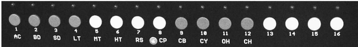
The LED over the current pattern blinks to show that it is active. When a new pattern is selected, the corresponding LED is lit, but stays solid. After the last step of the current pattern, the sequencer switches to the newly selected pattern. Now the LED of the new pattern blinks.
