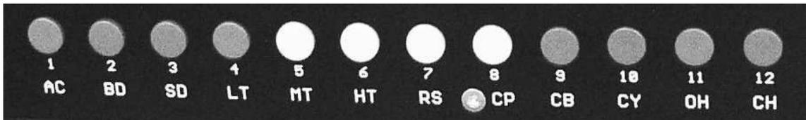
When the Inst./Select Button is held down, the currently selected Instrument is indicated by the LED above the corresponding instrument button. When the Inst./Select button is released, the pattern of this instrument is displayed by the LEDs over the Step Buttons (1-16)
