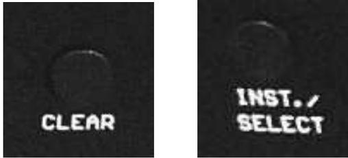
If the Clear Button and the Inst./Select button are held for a longer period, all instruments will be erased from the steps the sequencer passes through during the time the buttons are held.
