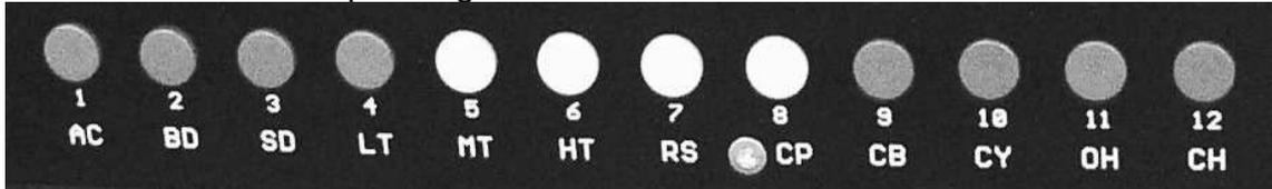
The instrument buttons (BD, SD, LT, ... ), write their instrument to the running pattern at the instant they are pressed. The accent button (AC), can be used to add an accent to the instruments programmed on a step. The LEDs over the instrument buttons indicate which instruments are programmed at each step. If you program the same instrument on a step more than once, it will not affect the pattern.
