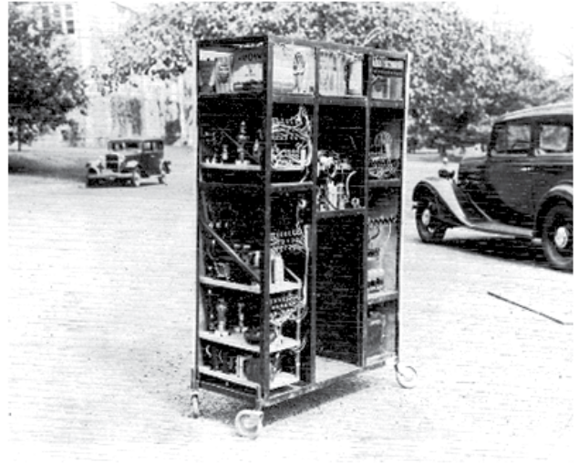
Schmitt's analogue computer "Nerve Axon Simulator" circa 1937
