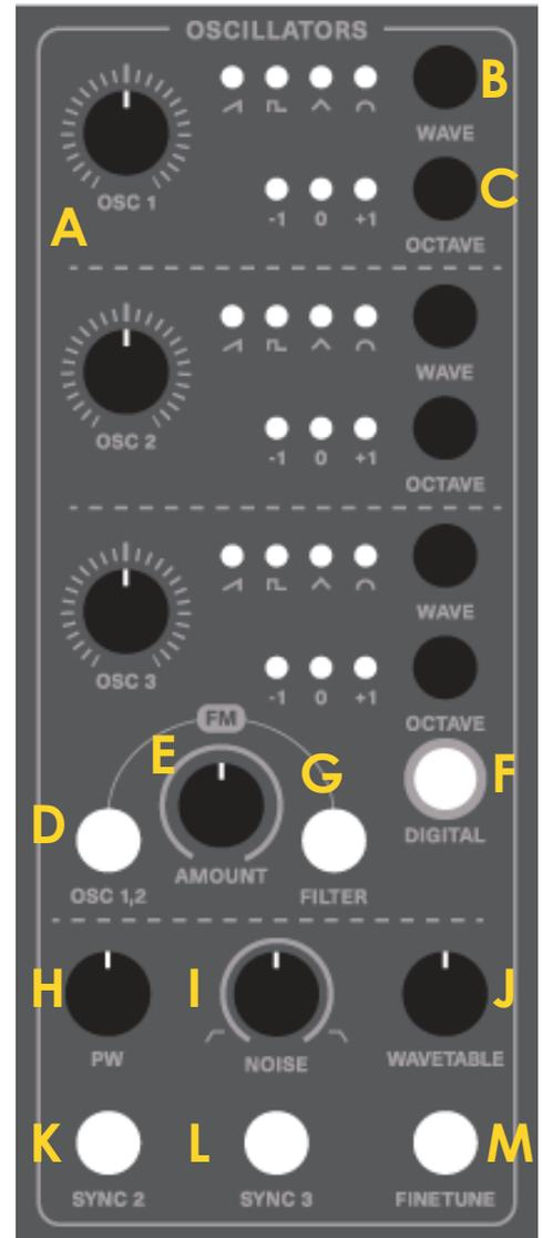
The **NOISE** knob (I) lets you mix a balance between brown noise (low-pass 6db/oct) and violet noise (high-pass 6db/oct). In the middle position it offers grey noise (notch filtered) equally mixing both the low-pass filtered noise and the high-pass filtered noise.
