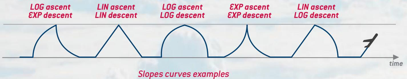
The CV Input for each Airplane's stage requires **3.5 mm mono plug (not stereo)** to function properly. The range of acceptable-voltage is  $\pm 5$  volts (10 Vpp). It's also possible to contol the shape of the slope (from exp-to-lin-to-log) instead of the time. By installing appropriate jumper settings (see the **Jumperization Chart**) the control of the input voltage is changed from 'control over parameter time' to 'control over parameter shape'.
