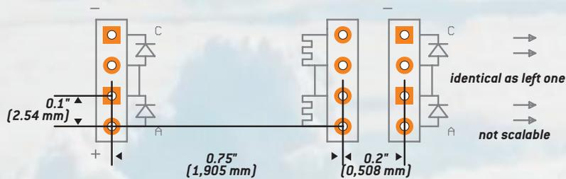
**Drawing of sockets for opto-couplers. View from the rear side of the Terminal module (bottom side of the PCB)**
