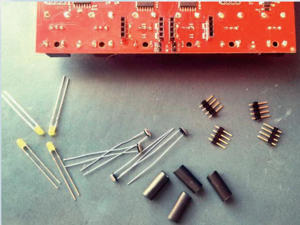
Same as in chapter 1 – you need to prepare 2pcs. of PLS-4 4-pin strips for each Gate. Additionally you need to prepare 2 pcs. of black 1cm length heat-shrink tube per each Gate.
