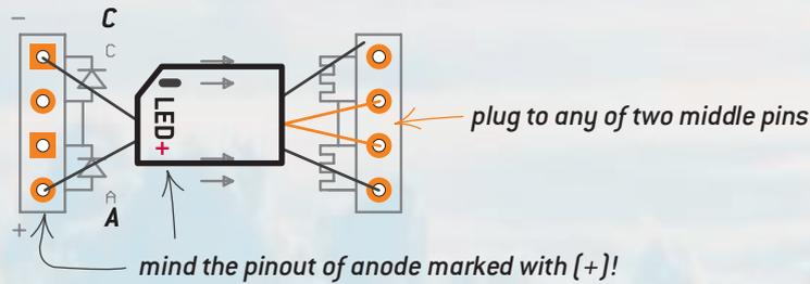
Before installing the opto-couplers you may want to cut their legs off to 1 cm length each and bend them 90° down to fit into socket. After installing new opto-couplers and checking the gates are working properly, you may apply a small amount of hot glue to the spots where the pins are inserted into the sockets to ensure the opto-couplers will stay there firmly.
