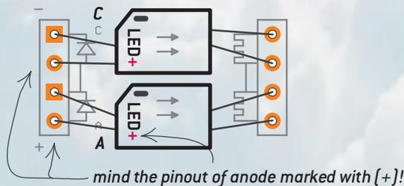
When installing one dual opto-coupler, the LED's pins should be connected to the most distanced pins marked **C** for cathode (shorter leg) and **A** for anode (longer leg). Dual opto-couplers have three pins. The side LDR's pins should be connected to the appropriate socket's side pins and the middle LDR's pin should be connected to any of two socket's middle pins:
