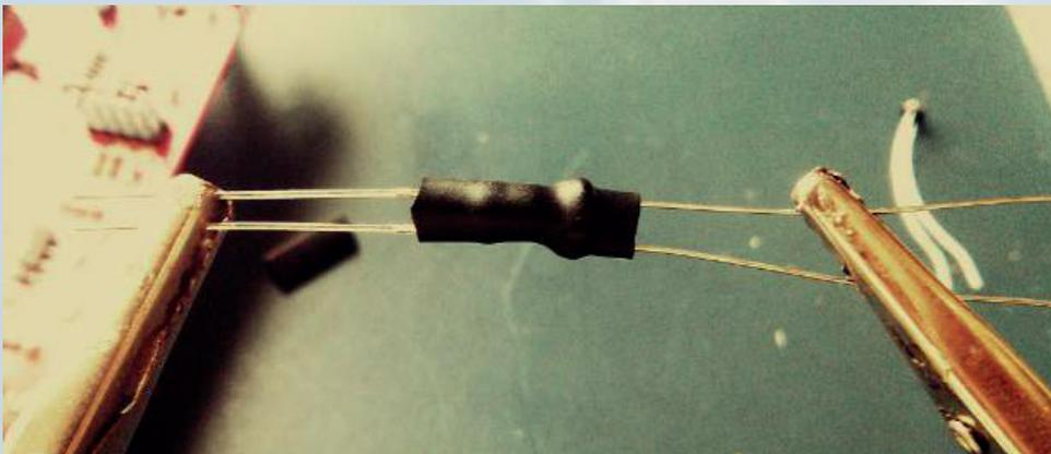
Put the vactrols on the IDC pins as on the picture below:
