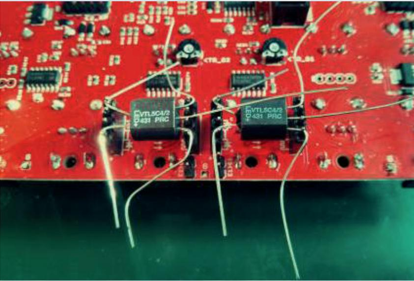
The factory vactrols should be put with their wires between the IDC pins with the graphics labeled upside up. The side with two LED pins (labeled as LED+ on the vactrol's case) should be on the left side of appropriate socket (LED+ on the vactrol should be on the same side where + is marked on the PCB).
