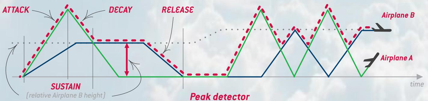
In **looping** mode both Airplanes work as **Voltage Controlled Oscillators** with **separately controlled** take off and Landingslope rates as well as **separately controlled** shapes of each slope. The take off and landing knob in far counterclockwise position, with no additional voltage applied, each stage has a durationof 1 ms or 500 Hz per whole cycle.
