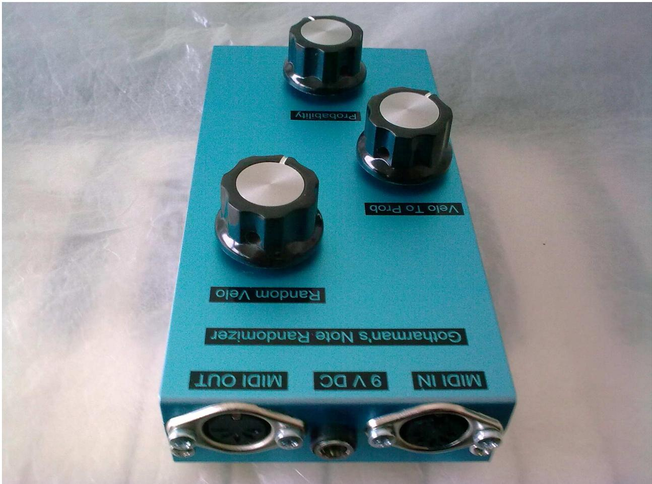
**MIDI IN:** Connect this to MIDI out from a MIDI device like a keyboard or a sequencer, that transmits MIDI note on's and off's.
