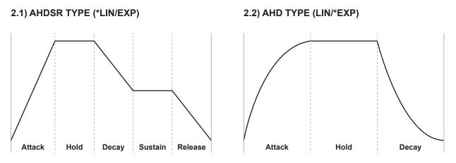
AHDSR is the ADE-51s standard, 5-stage envelope type, generated by a gate signal. A 3-stage AHD envelope can also be generated using the Trigger input where the time of the total envelope is set by the length of each stage and is independent of the Trigger/Gate length.
