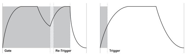
The AHDSR envelope type can be re-Triggered at any stage after Hold. The envelope stages start again from the Attack stage at whatever level the envelope it is at when re-Triggered. When the initial Gate signal ends - the envelope enters the Release stage as normal. The AHD envelope type operates independently of Trigger/Gate length with all stage times set by the relative front panel controls.
