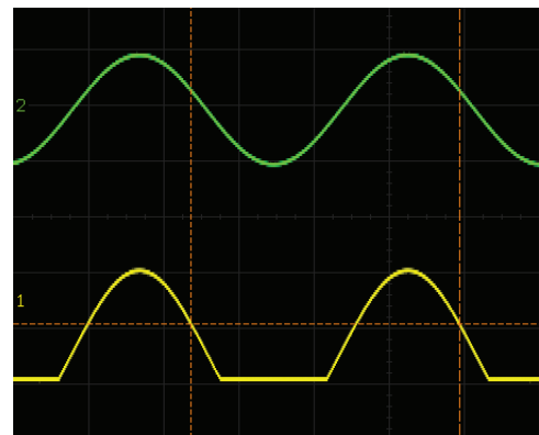
Fig. 2 - Asymmetric Distortion of a +/-5V Sine wave
