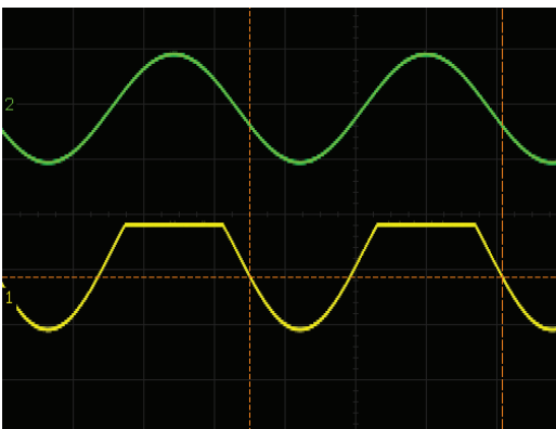
Fig. 1 - Asymmetric Distortion of a +/-5V Sine wave
