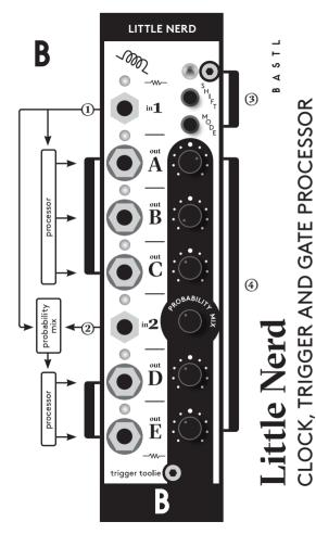
littleNerd is a trigger and clock manipulation module which tries to be able to do everything you have ever imagined and wished to do with trigger or clock signals in your modular in only 6 HP.
