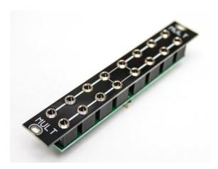
Thread the nuts onto the jacks and finger tighten them. Be careful not to pull the jacks out of the board during this operation or you'll have to start over.
