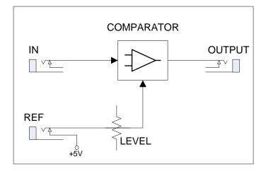
This diagram shows the comparator operation. The output is high when the IN signal exceeds the REF level.
