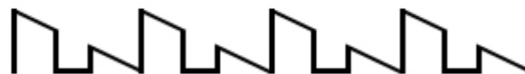
Envelope shape when accents are triggered from gates or triggers that are too short. ENV DECAY partially works.
