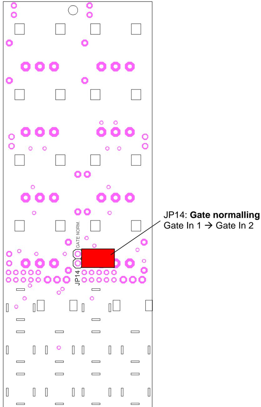
JP14 is an horizontal (lying) jumper and is located on the lower board. To remove or install this jumper a suitable tool has to be used (e.g. a small plier) because it's between the two boards. One may also remove the upper from the lower pc board for easier access. For this the mounting screw at the top of the board has to be removed and the upper board removed from the lower board by pulling out the two 10-pin connectors.
