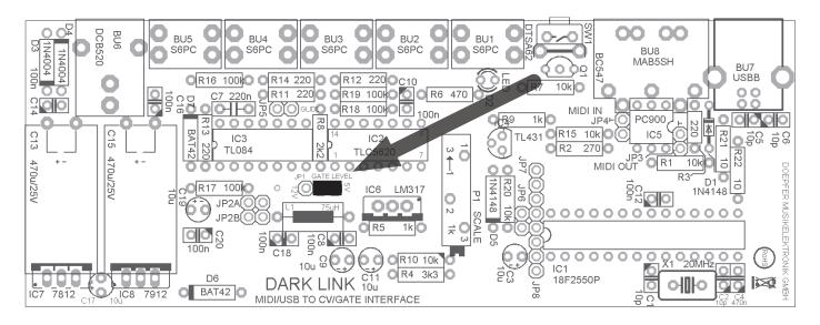
Jumper (JP1) position for 12 Volts trigger (middle and leftmost contacts):
