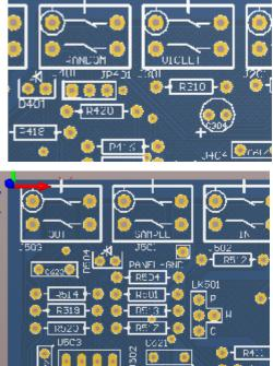
The SAMPLE connector is normalised to the RANDOM output of the NOISE section while the IN connector is normalised to one of the noise section outputs selected by LK501 (W=White, P=Pink, C= VIOLET. Inserting a jack in to any of these connectors will allow an external signal to be used instead.
