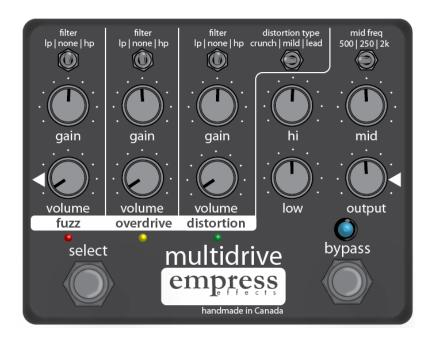
Set the knobs and switches to match the picture above. If the blue bypass LED is not already lit, press the **bypass** switch to engage the Multidrive. Now bring up the individual fuzz, overdrive and distortion values to taste. Rock out!
