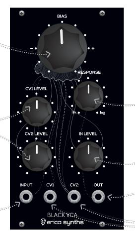
Smoothly fade from linear to more punchy logarithmical response modes. This knob is assigned to CV2 only
