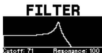
Figure 11: Filter response visualization: Cutoff and Resonance settings.
