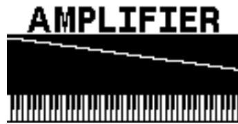
Figure 13: Amplifier keyboard tracking: This setting adjusts the amplitude response based on the pitch of the played notes, allowing higher notes to be louder or softer relative to lower notes.
