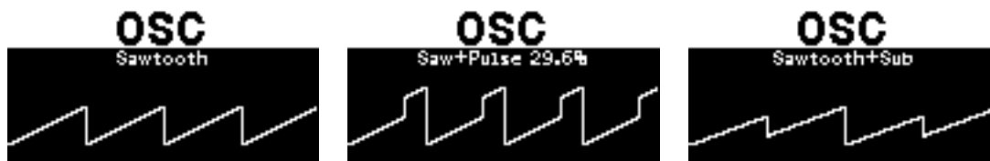
Figure 10: Oscillator waveforms: Sawtooth wave alone, mixed with pulse, or with sub-oscillator.
