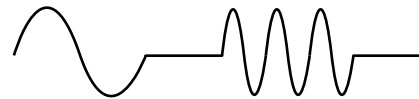
Fig. 2. Two pulsarets: one with a cluster value of 1, and the other with a cluster value of 3.
