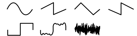
Fig. 3. Shape morphs between 7 waveforms: sine, up ramp, triangle, down ramp, square, noisy square, white noise.
