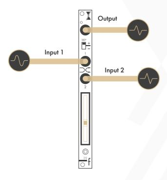
Attenuator: If a signal is present at Input 1 only and the Polarity Switch is in the up position, the module acts as an attenuator. When the Fader is in the up position, the signal present at Input 1 will pass to the Output. Moving the Fader downwards attenuates the signal present at Input 1 down to 0V at the lowest Fader position.
