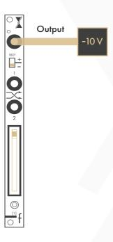
**Unipolar Positive DC Offset Crossfader:** If a signal is present at **Input** 2 only and the **Polarity Switch** is in the up position, the module acts as a unipolar positive DC offset crossfader. When the **Fader** is in the up position, the **Output** will pass +10V. Moving the **Fader** downwards crossfades from +10V to the signal present at **Input** 2.
