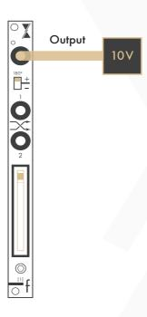
Unipolar Negative DC Offset: If no signal is present at the Inputs and the Polarity Switch is in the down position, the module acts as an unipolar negative DC offset. When the Fader is in the highest position, -10V is generated at the Output. Moving the Fader downwards attenuates the DC offset down to 0V at the lowest Fader position.
