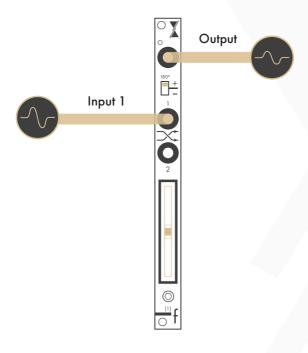
Attenuverter: If a signal is present at Input 1 only and the Polarity Switch is in the down position, the module acts as an attenuverter. When the Fader is in the up position, an inverted version of the signal present at Input 1 will pass to the Output. Moving the Fader downwards, attenuates the inverted version of the signal present at Input 1 down to 0V at the lowest fader position.
