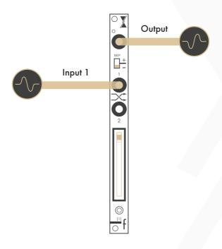
Unipolar Positive DC Offset: If no signal is present at the Inputs and the Polarity Switch is in the up position, the module acts as an unipolar positive DC offset. When the Fader is in the highest position, +10V is generated at the Output. Moving the Fader downwards attenuates the DC offset down to 0V at the lowest Fader position.
