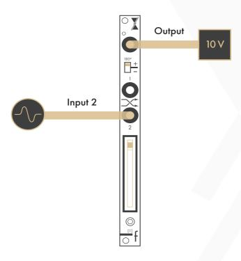
Unipolar Negative DC Offset Crossfader: If a signal is present at Input 2 only and the Polarity Switch is in the down position, the module acts as a unipolar negative DC offset crossfader. When the Fader is in the up position, the Output will pass -10V. Moving the Fader downwards crossfades from -10V to the signal present at Input 2.
