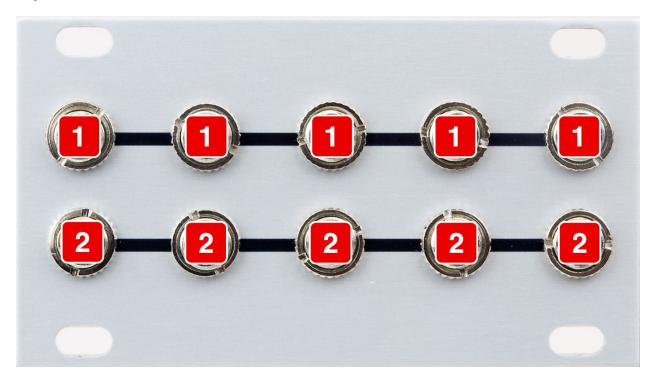
Mult 1U is a dual 5-way passive signal multiplier. A signal multiplier takes one input signal and routes it to multiple outputs simultaneously. For example, you might want a keyboard's gate CV to trigger two different envelopes — one to control volume and the other to control filter frequency. In addition, you might also want each key press to reset the phase of an LFO, which controls some other parameter, such as Pulse Width modulation on your oscillator.
