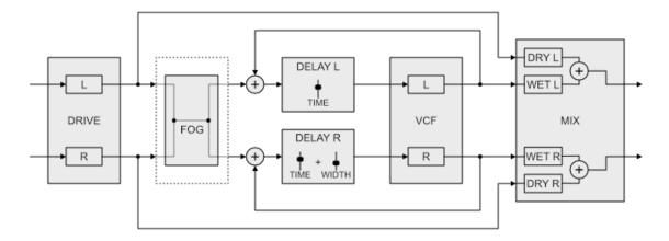
DLY (mid): Fog is positioned after the delay circuit, but before the MIX, meaning it
