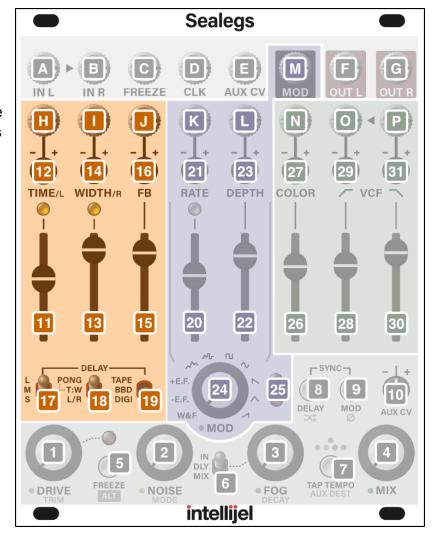
When un-sync'd, and free-running, the slider works over a range of 3.125 ms - 93.75 ms; 50 ms - 1.5 s; or 200 ms - 6 s, as set with the **TIME RANGE** [17] switch.
