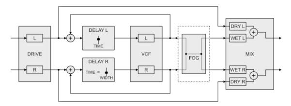
If ALT FB CROSS [8] is enabled, then crossing the feedback sends the output of the Right delay back into the Left input, and vice versa, creating the following routing:
