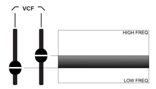
NOTE: Because both filters close at 6db/octave, frequencies that exceed the cutoff settings will still pass through, albeit at an attenuated level. Consequently, positioning the **HIGHPASS FREQ [28]** slider above the **LOWPASS FREQ [30]** slider will not result in a total cessation of sound, but rather an attenuated reduction of overall level, centered around the midway point between the two sliders.
