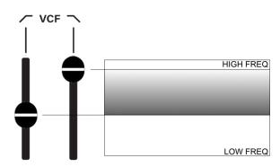
Lowering the **LOWPASS FREQ [30]** slider removes high frequency content from the signal. As a result, the position of both sliders gives a visual representation of the frequency band passing through the filter.
