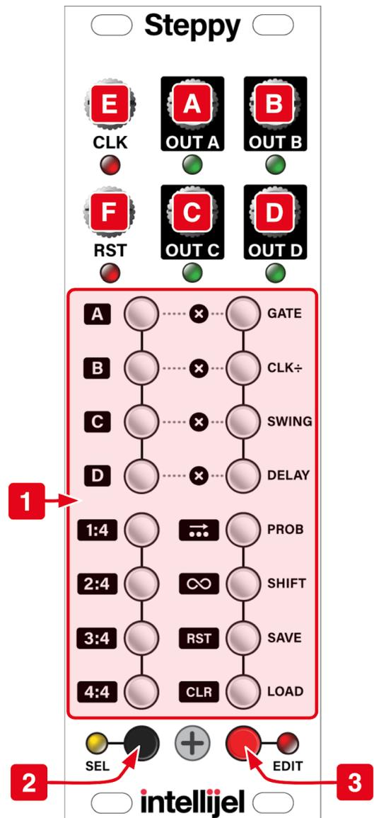
Hold the **SAVE RST** button on boot up to toggle between RUN and RESET modes (the setting is saved across boots). On the SELECT page, you'll see the **SAVE RST** button light **yellow** if RUN mode is enabled.
