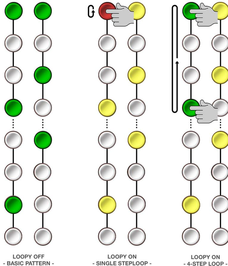
If Loopy(  $\infty$  ) is active, pressing *one* button loops playback of that single step, repeating it over-and-over for as long as you hold the button (as seen in the middle example, above). The button is **red** because red indicates the current playback position, which is endlessly repeating on a single step. The other buttons are **yellow** indicating they are programmed into the pattern, but are not within the currently playing loop.
