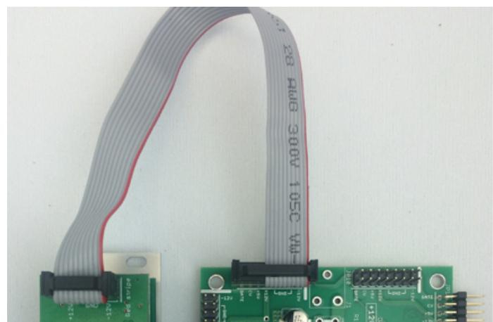
After you have confirmed all the connections, you can reconnect the power cable and turn on your modular system. You should immediately check that all your modules have powered on and are functioning correctly. If you notice any anomalies, turn your system off right away and check your cabling again for mistakes.
