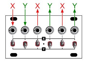
In this illustration, we see that jacks 1, 3, and 5 are switched to the X bus, while jacks 2 and 4 are switched to the Y bus. Jack 6 is switched off (middle position), so it carries no signal.
