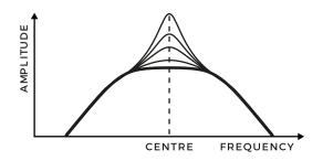
At sufficient filter width and resonance levels, self-oscillation will be achieved, turning the filter into a sine wave VCO.
