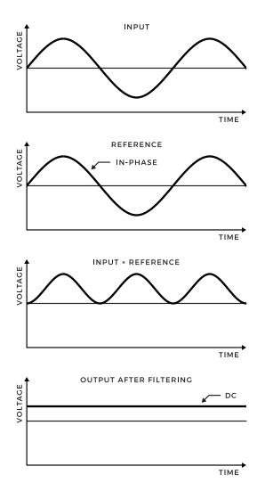
As can be seen, the result of the multiplication process is a sine wave at double the input/reference frequency, with a DC offset. After filtering, only the DC voltage remains, which is equivalent to one quarter of the input AC amplitude in V<sub>pp</sub>.
