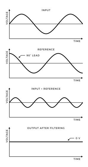
In this case, the multiplication result no longer has a DC offset, so the output voltage after filtering is 0 V, highlighting the phase-dependency property of the synchronous detection process.
