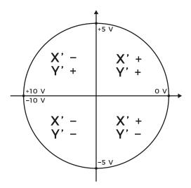
For example, if X' and Y' are both positive and equal in voltage, this represents a phase angle of 45°, corresponding to a phase output voltage of +2.5 V.
