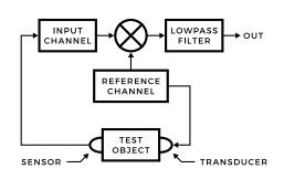
In Collide 4, the reference channel is simply called the oscillator, and it consists of a quadrature VCO. This means that its two outputs (I and Q) are identical sinusoidal signals, with identical amplitudes, but a fixed phase separation of 90°—or, in other terms, a sine and cosine output pair.
