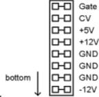
The bottom is the edge of the PC board
