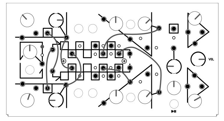
*Phasing Patterns* The registers here are looping data from the bit outputs back to the data input. Enter data using the red data + button on each sequencer.
