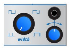
The **Width knob** controls the duration (duty-cycle) of the generated pulses. It is set in percentage of the main clock cycle. So when the clock rate changes the pulse width will follow accordingly. The smallest pulse width is 1% of the duty cycle, the maximum width is 99%.
