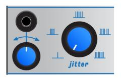
The **Jitter knob** adds a time offset (time delay) to each of the six **Pulse output** with respect to the main clock (external or internal). This jitter could be generated both before/after relative to the main clock tick. At each input clk edge the alogithm compute the next coming clock jitter combinaison to be applied. So always expect 1 clock cycle delay to get the result
