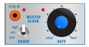
The **Rate** controls the period of the internal clock generator of the module. It works together with the clock selector switch [LOW EXT HIGH] to reach a wide range of periods from 2ms to 5s. The associated **Rate LED** helps to monitor the actual rate.
