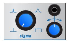
The **Sigma knob** adjusts the width parameter of the Gaussian distribution.
