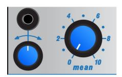
The **Mean knob** setting corespond to the mean value of the distribution of outgoing CV levels. It can be interpreted as a global offset of the six **CV outputs** level around which gaussian voltage variations will be added.
