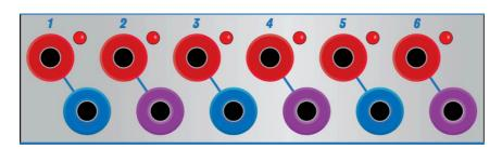
For each of the six **PULSES Outputs**, there is a corresponding control voltage **CV Output**. The CV levels are changing synchroneously to the corresponding pulses rising edges. The algorithm used to generate these control voltages is using a gaussian distribution controlled by the knobs sitting on the top of the module pannel. The pulse LEDs let you monitor the pulses width and/or when the CV value is being updated.
