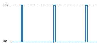
Figure 8: Typical Trigger Signal
