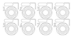
Phase spread, vari-speeded copies of the input signal. +/-10Vpp
