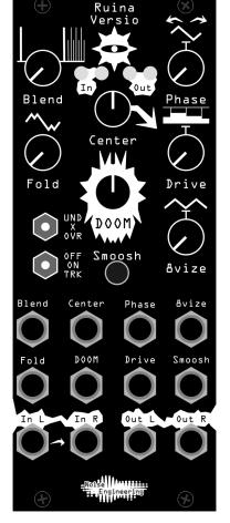
Start by playing with Fold, Doom, Drive, and 8vize: these are the main controls for the four types of distortion on RV.
