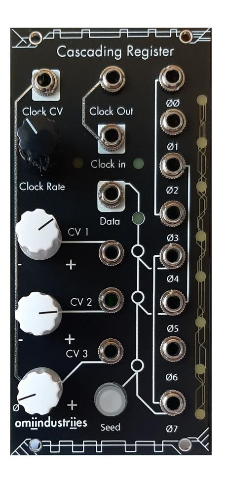
The Cascading Register from omiindustriies is a source of pseudo-random voltages and gates using an eight-bit shift register. It takes inspiration from digital shift registers, runglers, linear feedback shift registers (LFSR), and analog shift registers.
