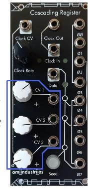
The CV outputs come from the first four, the middle four, and the last four stages of the shift register which creates three copies of a CV signal, shifted by two clock pulses. The three white knobs control the amplitude of the CV outputs, allowing you to fine-tune the amount of modulation. CV1 and CV 2 include attenuverters (bipolar level control), while CV3 uses an attenuator (unipolar level control).
