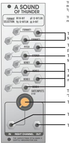
The new SOUND OF THUNDER expands the capabilities of your Tyme Sefari base unit. To install, simply connect the short ribbon cables labeled "THUNDER" and "THUNDER2" to the corresponding locations on the rear of the Tyme Sefari.
