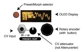
determine if all panel settings are affected by the preset change, or just the waveform selection controls. The CV input and attenuator knob just below the display also changes the active preset. The behavior of the CV and knob is defined in the GLOBAL OPTIONS menu with the CTL option.
