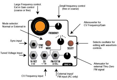
The "FM" input provides audio-rate, thru-zero frequency modulation of the oscillator signal. It only accepts audio-rate signals. When the OSC MODE button is pressed the Piston Honda enters External In mode, this input provides the signal to be dynamically waveshaped through the selected wavetable (instead of using the internal oscillator) When active, "Ext" will be visible over the waveform display.
