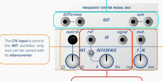
**FM** receives an audio input and can be applied to **INT**. The **amount** of modulation is determined by the **attenuator knob**.
