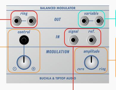
The bottom MODULATION section applies to the "variable" double output.
