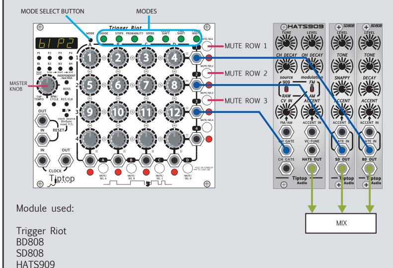
1. Lets start again by connecting OUT 1 to BD808, OUT 2 to SD808 and lets patch OUT 3 to Open Hi-Hats 909. Lets press and hold RST/CLR button to make sure we start from scratch...
