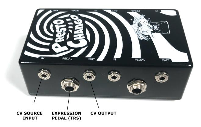
The Presto Chango is an adapter box that provides the use of up to 4 standard expression pedals, like the Moog EP2 and EP3, with eurorack jack format modular synths. The Presto Chango has been tested to work with Moog EP2 and Moog EP3 Pedals, which have TRS audio connectors. Others with a TRS connector may work, but have not been tested. Expression pedals with only a TS style connector will not work with the Presto Chango.
